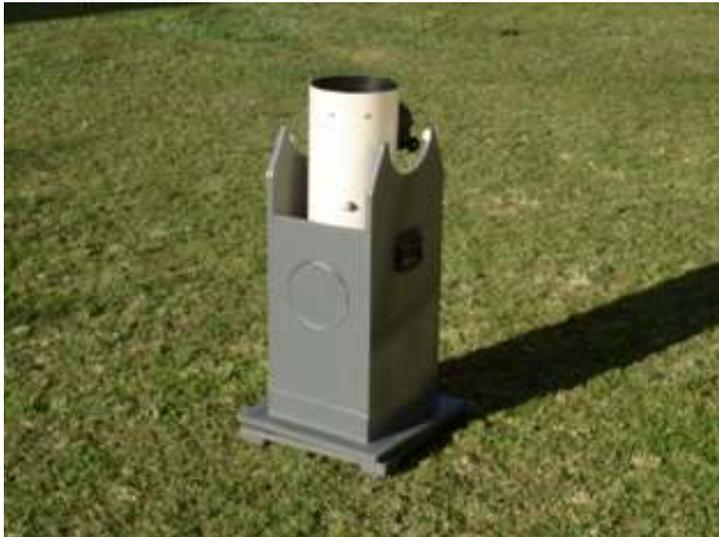
The telescope its self had been designed to be compact. I had incorporated a few ideas that I felt would make this scope easier to transport and store than the f9. Firstly I designed the base so that the tube could rest inside it for storage. The round trunions could pass through a hole in the rocker box allowing the minimum area to be filled when stowed. I also realised that such a small
